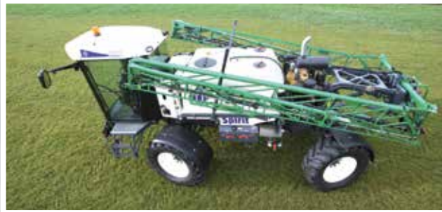
Simple design with rear mounted CAT engine power pack
