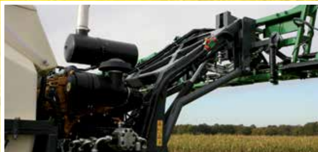
Pantograph arms for precise spraying height
